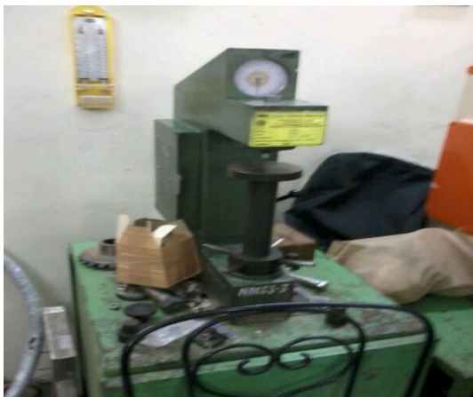
Fig: 3. RESULT: The Rockwell hardness test gave 25-26 HRC
